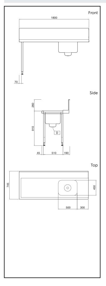
Handling System for Hood type Pre-wash Table with 500x400 Bowl and Strainer Left to Right, 1800mm
